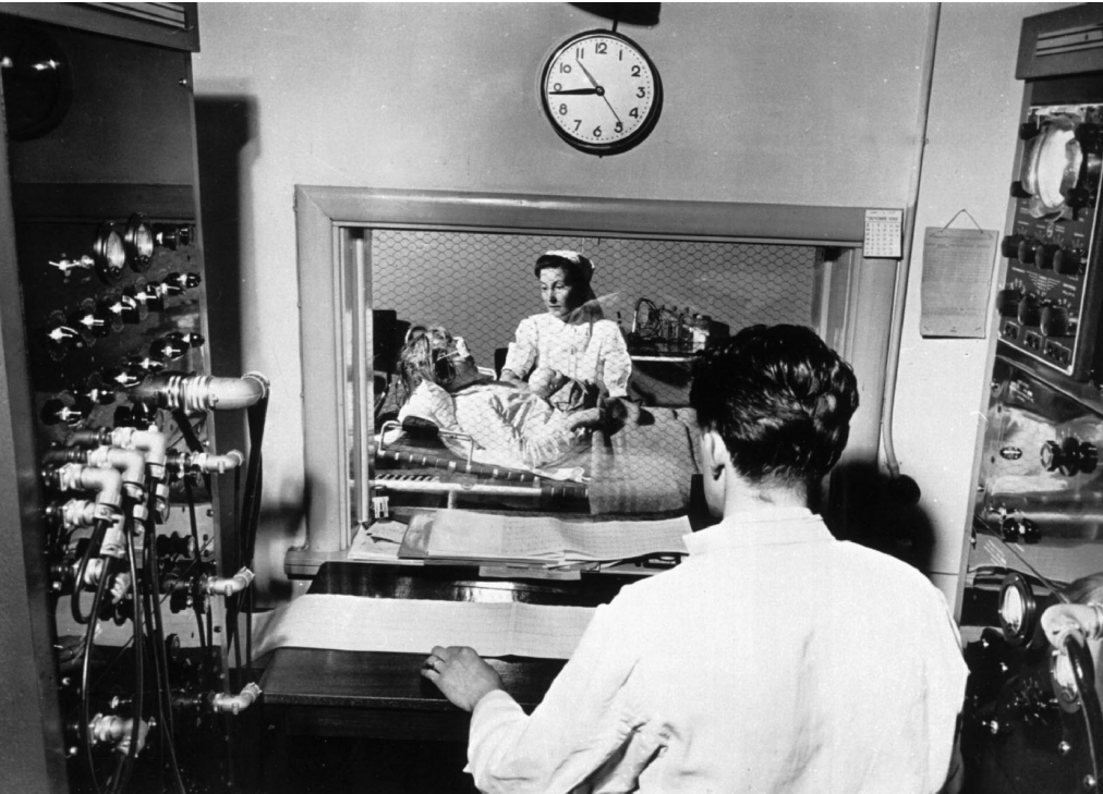
Figure 3. EEG registration in 1949: the technician is sitting 'in' the EEG machine (an Offner Dynograph). The same machine was used for EMG. For this application an oscilloscope was added (top right).
